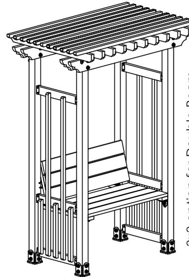
2x2 option for Double Beam with Timber Bolts & Bench
